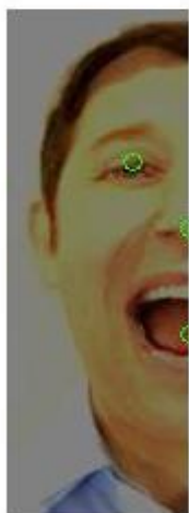
Fig. 7 Average Half Face with detected feature points of eye, nose and mouth
